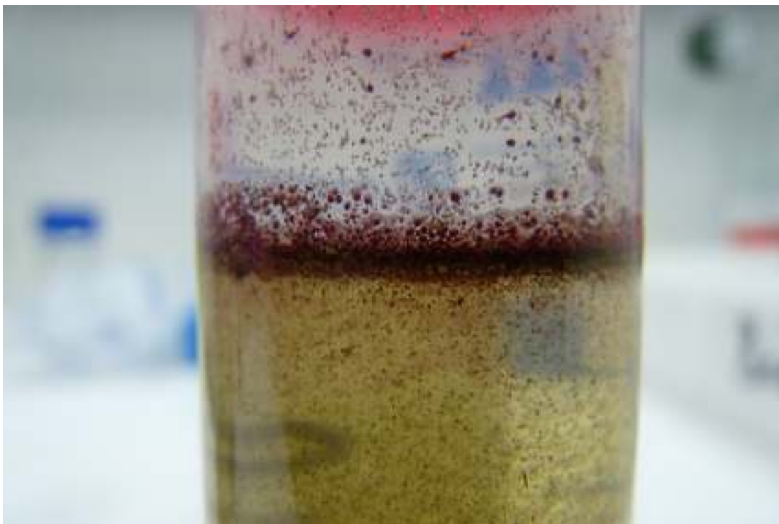
Figure 8: Stained foraminifera floating on top of the Sodium Polytungstate solution.
