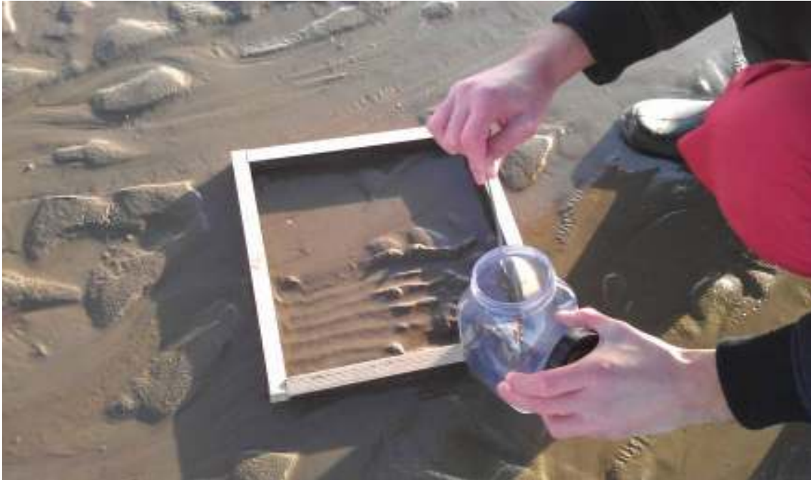
Figure 4: Surface sediment collection (~0.5 to 1 cm).
