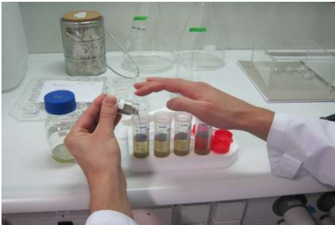
Figure 7: Sediment samples mixed with Sodium Polytungstate.
