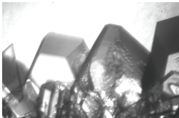
Figure 2. Magnesium sulfate hydrate crystals at a pressure of 249 MPa and a temperature of 242.5 K.
