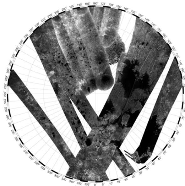
Fig. 1: Polar stereographic projection (65 – 90 N) of Cassini SAR imagery, consisting of imagery obtained during T16, 18, 19, 25, 28, 29 and 30 fly-bys. Longitude given in non-standard degrees E.
