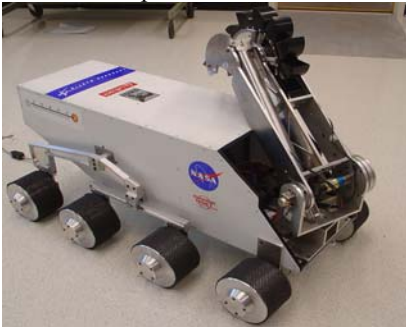
Figure 1. Colorado School of Mines' prototype lunar bucket wheel excavator.
