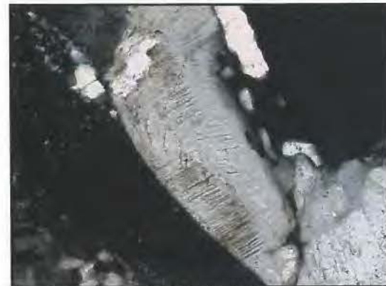
Fig.4: Two sets of PDFs in feldspar grain. Cross polarized light, width of view field 0.52 mm.
