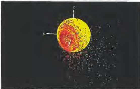
Figure 1. Simulation timestep ( t = 0.58 hrs) for a 1.45 \times 10^{29} J, 10 km/s, 45^\circ impact. Color represents internal energy
