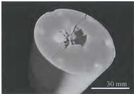
Figure 2. CT reconstruction of target surface viewed from above/oblique. Stainless steel projectile, 2mm diameter, shot G160606#1. Note extensive spall detachment of segments bounded by radial fractures.
