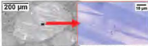
Figure 4: Plastic deformation:-kink bands and planar features (high pressure slow compression experiment)
