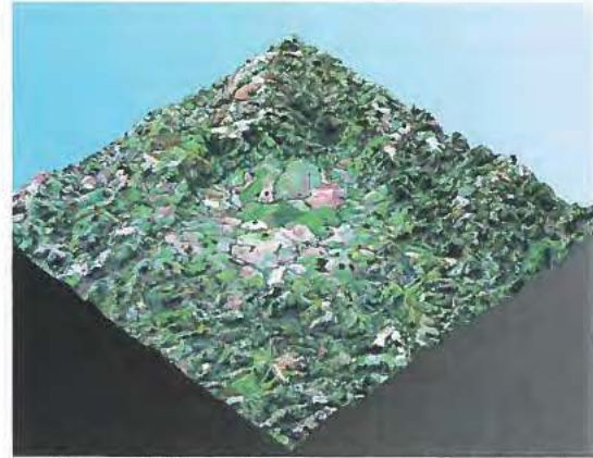
Figure 3. Vista Alegre in a perspective view using Landsat ETM+ image draped over Shuttle Radar Topographic Mission (SRTM) digital elevation model.
