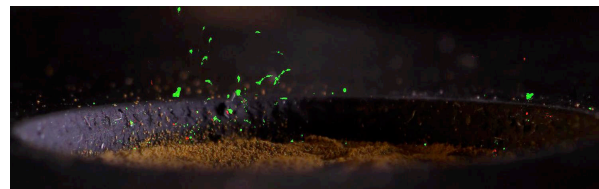
Figure 1: Trajectories (highlighted in green) of dust particles (Mars simulants, 38 – 48 microns) hopping off the surface that was exposed to plasma and 140 eV primary electrons. The surface morphology became smoothed after dust redistribution.
