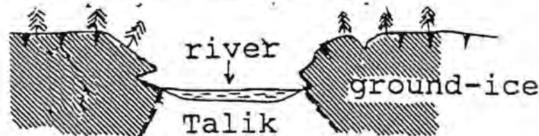
Fig. 1: Thermal erosion in Siberian rivers.
