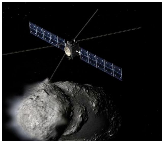
Figure 2. CORE acquires a dense network of radar echoes from polar orbit to obtain a 3D 'CAT scan' of the comet nucleus. It utilizes mature techniques of planetary radar, in a 3D geometry that leads to high definition migration imaging and tomography.
