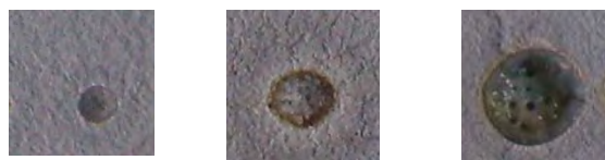
Figure 1. Image of artificial fulgurite; left: irradiated 5s at 8W; middle: irradiated 30s at 8W and right: irradiated 5s at 40W
