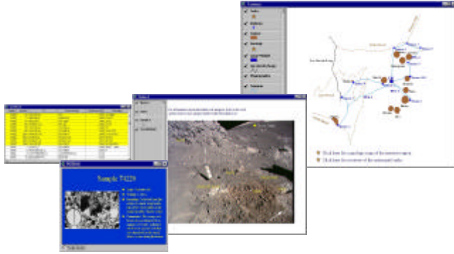
Fig. 2. An example of the Taurus-Littrow GIS. The user can select a site and search for information on samples collected, data acquired, sample location, size, and more.
