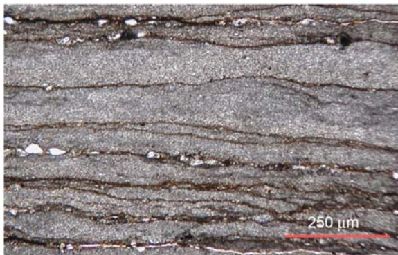
Figure 1: Laminated basal Todilto; fine-grained calcite with detrital quartz (clear grains). Minor gypsum and kaolinite are associated with dark, bituminous bands.
