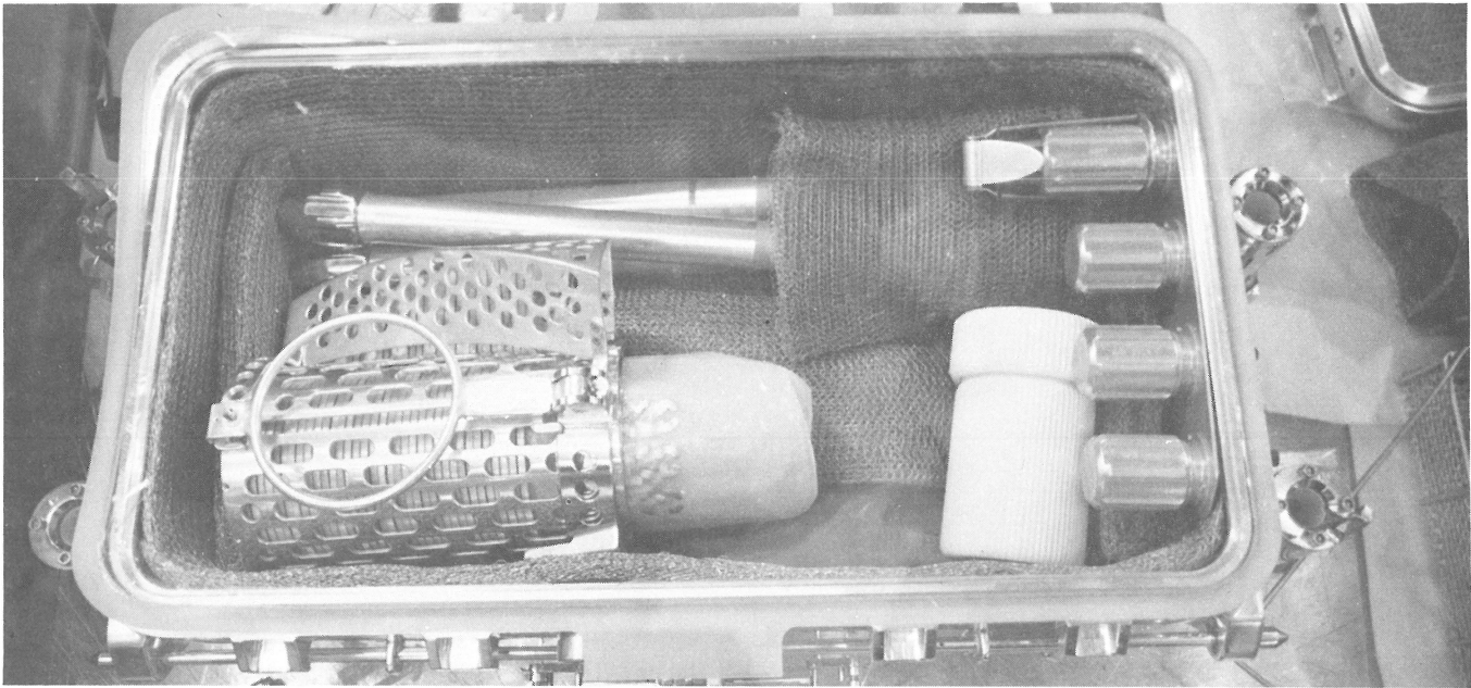
Fig. 71. Apollo 14 Lunar Sample Return Container prior to flight packed with round documented sample bags, 2-cm diameter core tubes, core tube caps, and Magnetic Shield Sample Container (believed to be the white cylinder) (NASA photo S70-29818).
