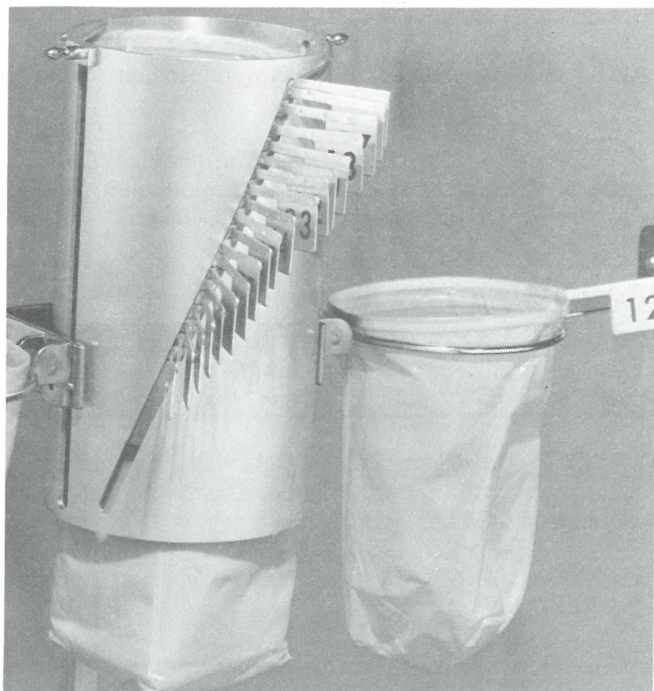
Fig. 79. A proto-type of the 35-bag dispenser for the cup-shaped documented sample bags showing the aluminum band re-inforcing for the top of the bag (NASA photo S68-54935).
