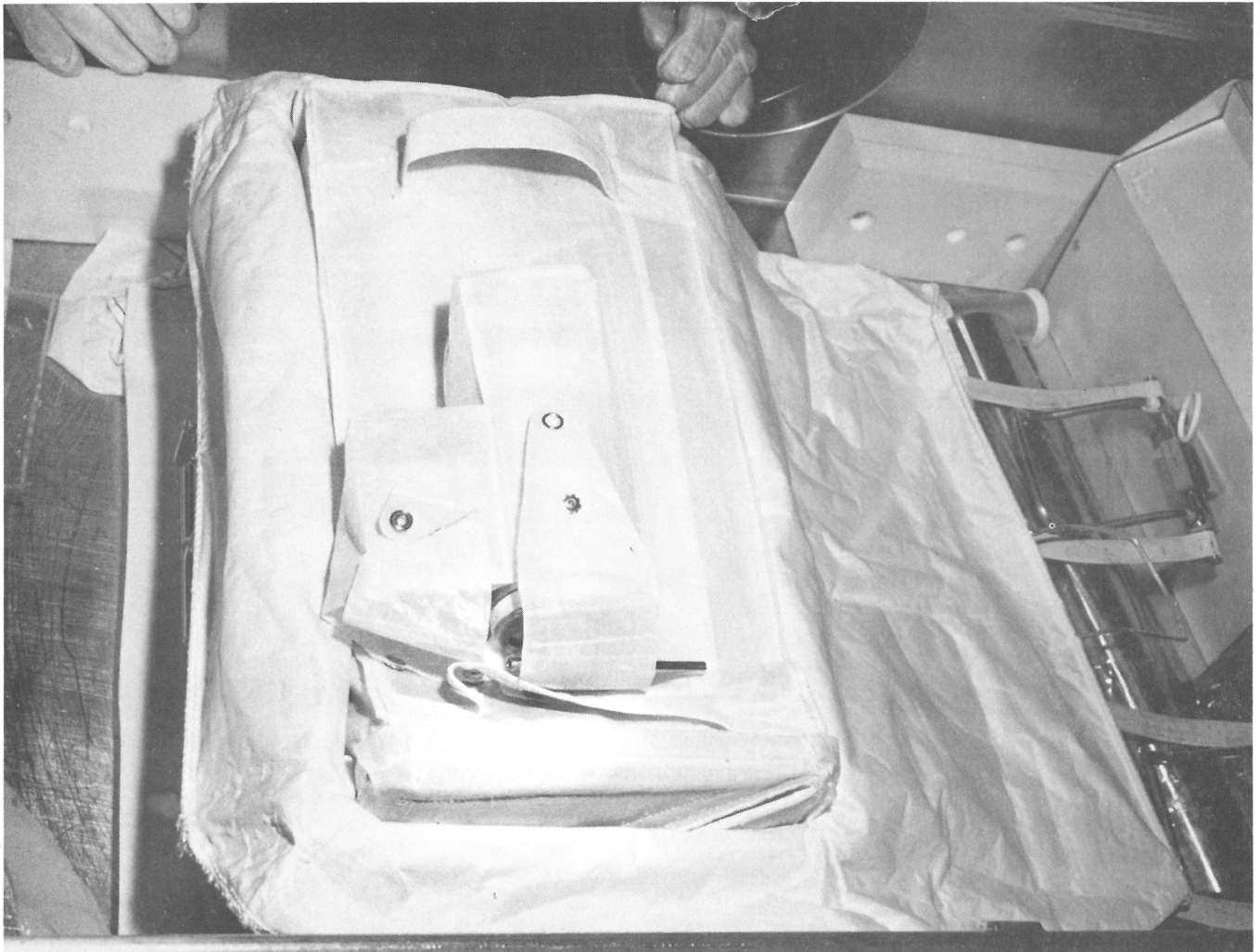
Fig. 96. Sample Collection Bag packed into Apollo Lunar Sample Return Container before the Apollo 15 flight. The edges of the ALSRC are draped with white material similar to that of the SCB. The SCB is lying on its side with the lid toward the viewer. The exterior pockets containing a Special Environmental Sample Container and a drive tube cap dispenser are visible (NASA photo S71-36042).
