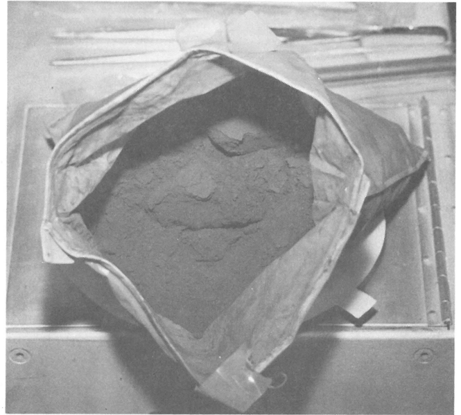
Fig. 83. Flat, rectangular documented sample bag opened in laboratory to show Apollo 17 soil 74220, weighing 1180 g. The aluminum rim holds the bag open (NASA photo S73-15561). S73-15061
