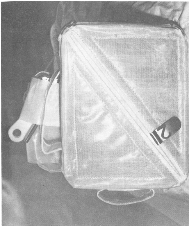
Fig. 98. Top of closed Sample Collection Bag The fabric texture and the diagonal slit through which samples could be dropped is visible. The white fabric in the background is part of the seal protector for the ALSRC (NASA photo S88-52673).
