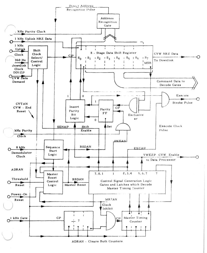
Figure 4-10 Control Logic 4-19
