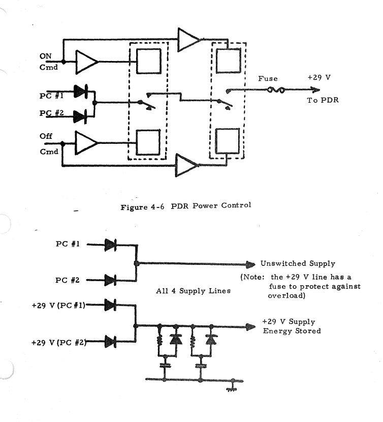
Figure 4-7 Data Subsystem Unswitched Supply Lines
