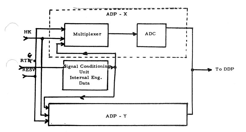
Figure 4-14 Analog Data Processor (ADP)
