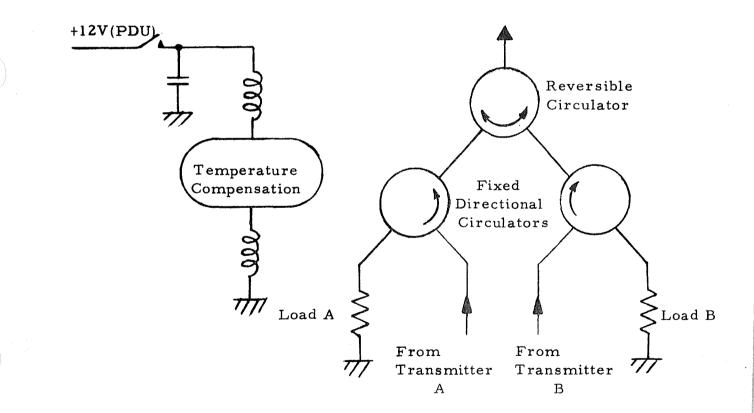
Figure 4-31 Circulator Switch Block Diagram
