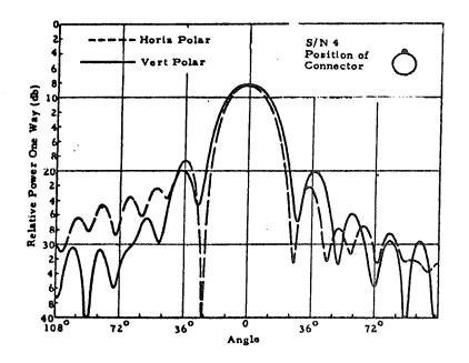
Figure 4-32 Typical Antenna Pattern, Transmit Frequency
