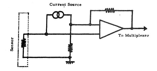
Figure 4-18 RTG Temperature Sensing Circuitry
