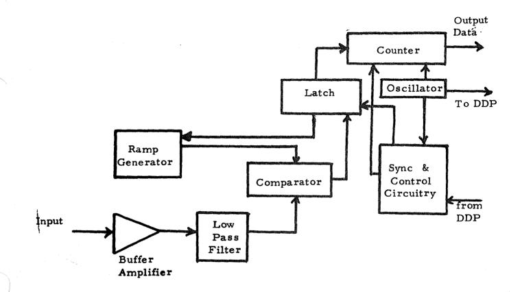
Figure 4-16 ADC Block Diagram
