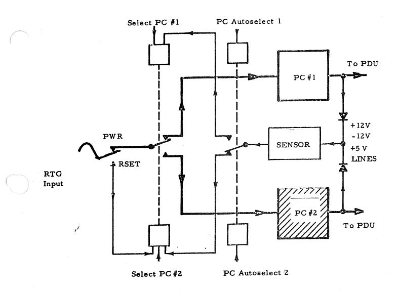
Figure 3-3 PCU Auto Switch Circuitry
