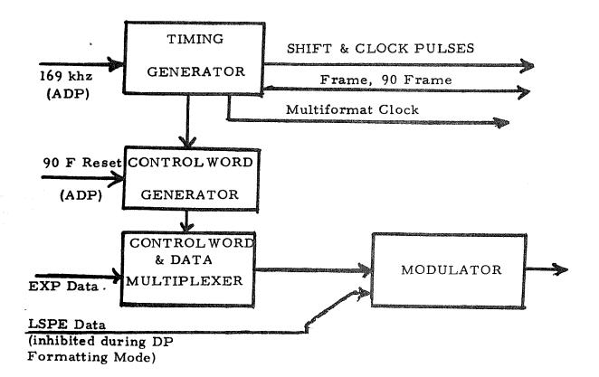
Figure 4-21 Timing and Control Word Generator
