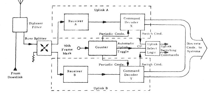
Note: Only Uplink A or Uplink B powered at any one time Figure 1-6 Array E Uplink
