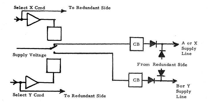
Figure 4-1. Transmitter/DDP Power Control
