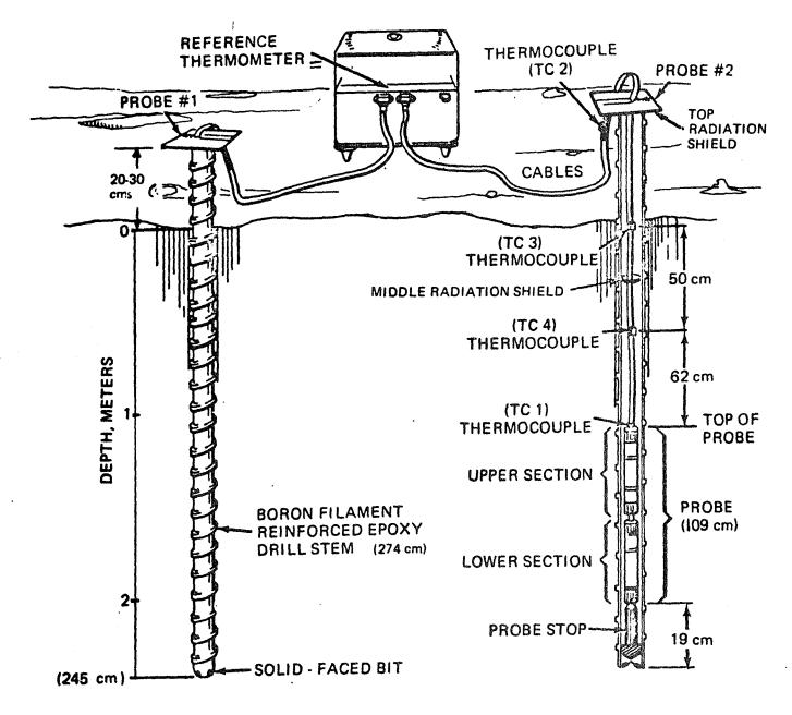
Figure 5-7 Heat Flow Experiment Deployed Configuration
