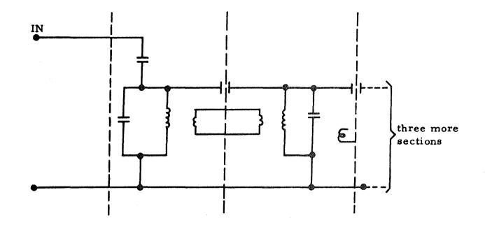
Figure 4-30 Bandpass Filter Equivalent Circuit
