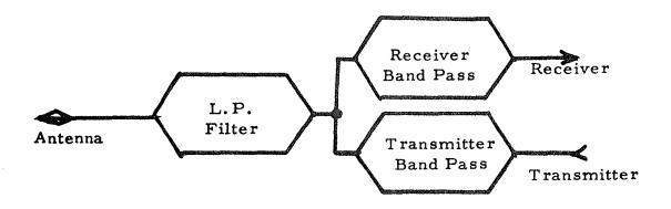
Figure 4-28 Block Diagram of Diplexer Filter
