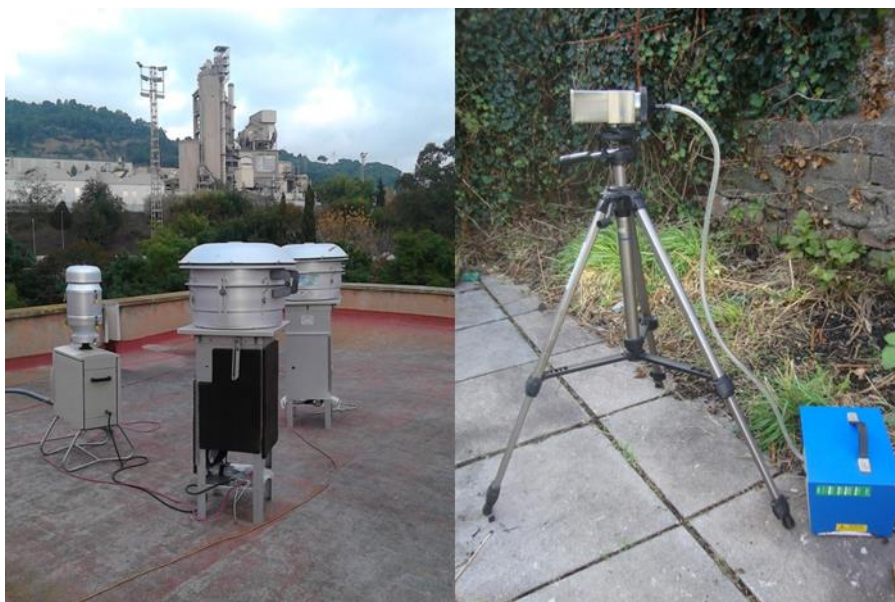
Figure 8: High volume TE-6070-DV (Tisch) and CAV-A/mb (MCV) samplers (left) and low volumen horizontal elutriator sampler (Negretti) (right).
