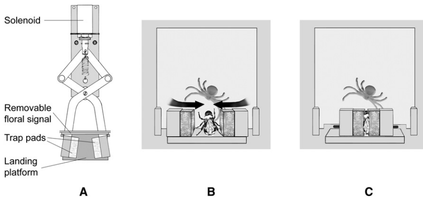
Figure 1. Schematic View of a Simulated Predation Attempt
