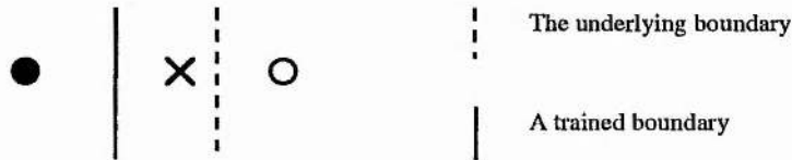
Figure 7.1. The cross indicates a pattern from the underlying problem which does not belong to the training set and is misclassified by the trained boundary.
