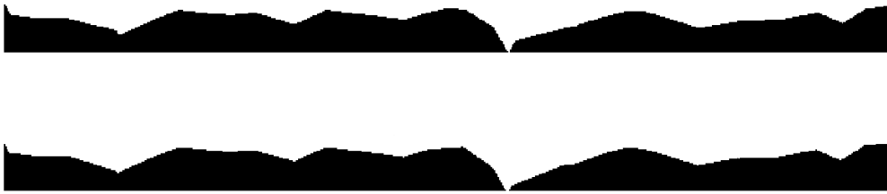
Figure 1. Simulated KMC (top) and GP predicted (bottom) deposition shapes for a lattice size of 650 atoms and 200 atomic layers.
