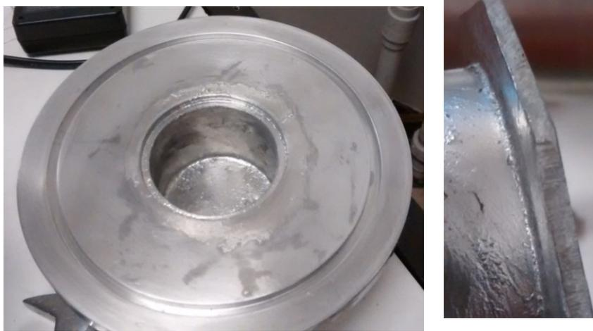
*Figure 5.40 – Vacuum side of the test flange and a close-up of the atmosphere side of the joint n.b jointing has not been polished*
