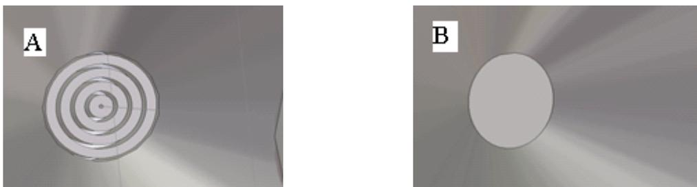
Figure 5.26 Hot cathode geometries: a) approximate spiral b) solid cathode.
