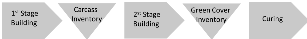
Figure 2 – Manufacturing stages and Inter stage inventory
