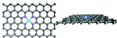
Fig. 10 Optimised structures (top and side view) of a structure resulting from the FeN 4 moiety embedded in an extended graphene sheet. Grey, blue and cyan spheres represent carbon, nitrogen and Fe respectively. Taken from Szakacs et al. 189 .
