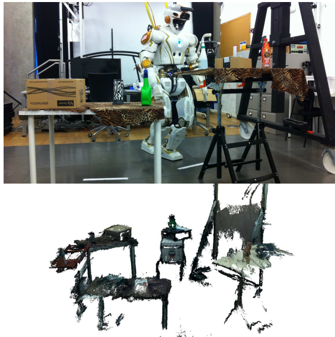
Fig. 1: Top: The NASA Valkyrie humanoid robot during operation in a laboratory environment. Bottom: stereo 3D reconstruction of a manipulation scene covering a 12m 2 area
