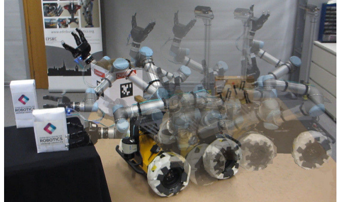
Fig. 1. The bimanual mobile manipulator executing a shared workspace task: model-free segmentation of target objects with automatic mobile base placement selection and navigation to place them in a bin. The system automatically adapts to various dynamic changes, including changing object and target locations during execution as well as scene monitoring for safe avoidance and replanning of motion to accommodate human operators.
