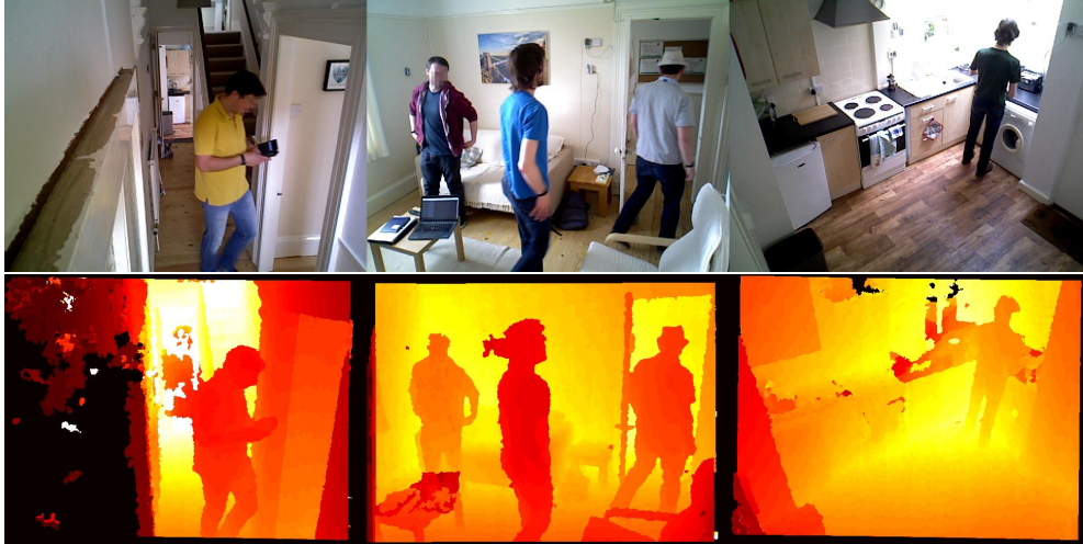
Figure 2. LIMA Dataset: Example RGB frames (top) and depth sensor measurements (bottom, darker is nearer) from cameras 1, 2, and 3 (left-to-right)
