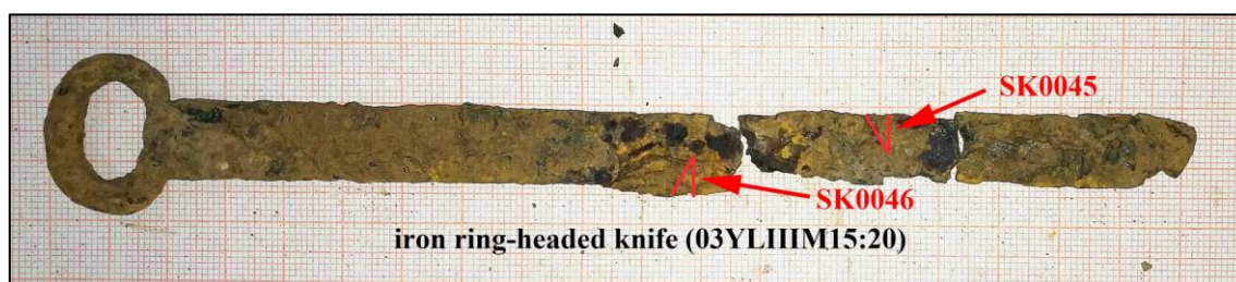
Fig. 5.105 Iron ring-headed knife (03YLHIM15:20) showing the sampling spot of SK0045 and SK0046 (source: author)
