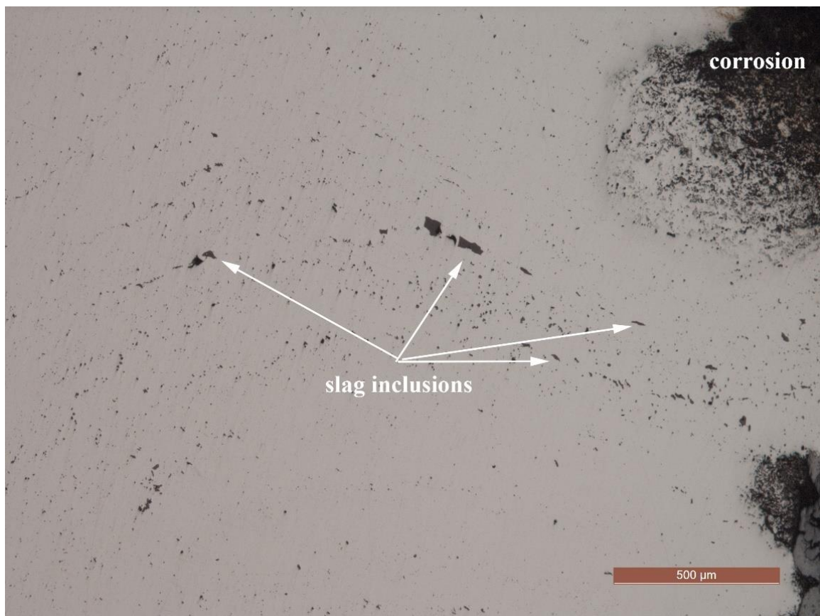
Fig. 5.42 Section from SK0012. Unetched, scale bar 500 \mu m (source: author)
