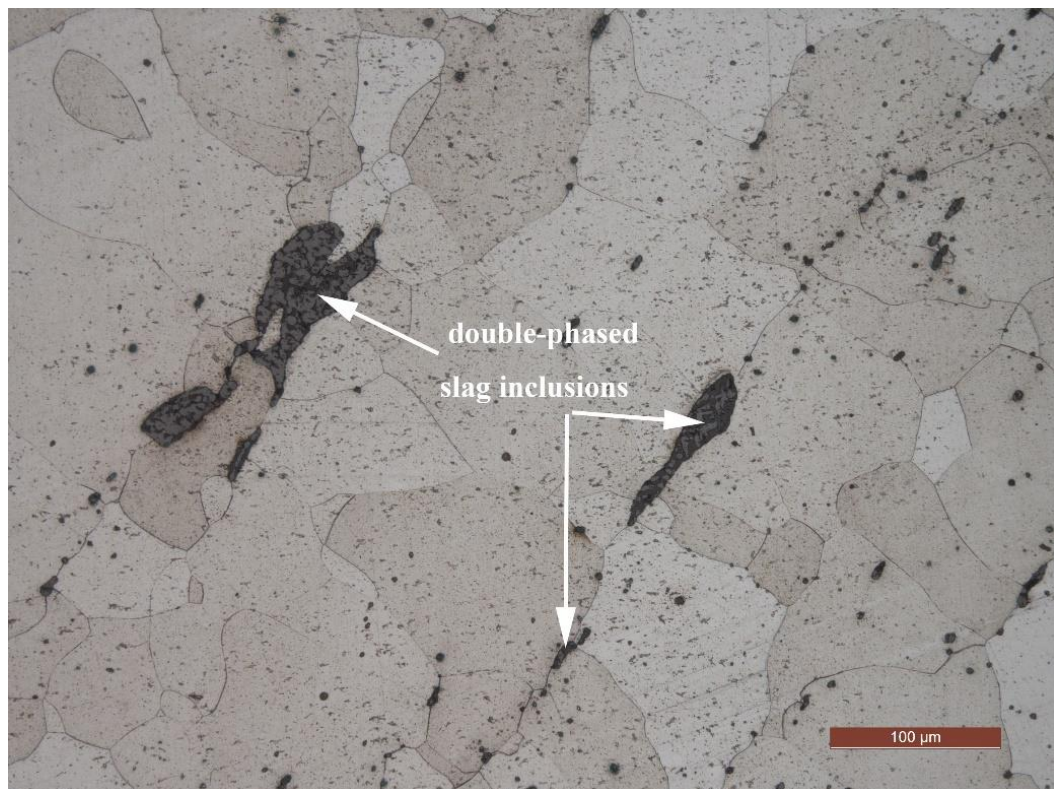
Fig. 5.25 Section from SK0005 showing the double-phased slag inclusions. Etch 2% nital, scale bar 100μm (source: author)
