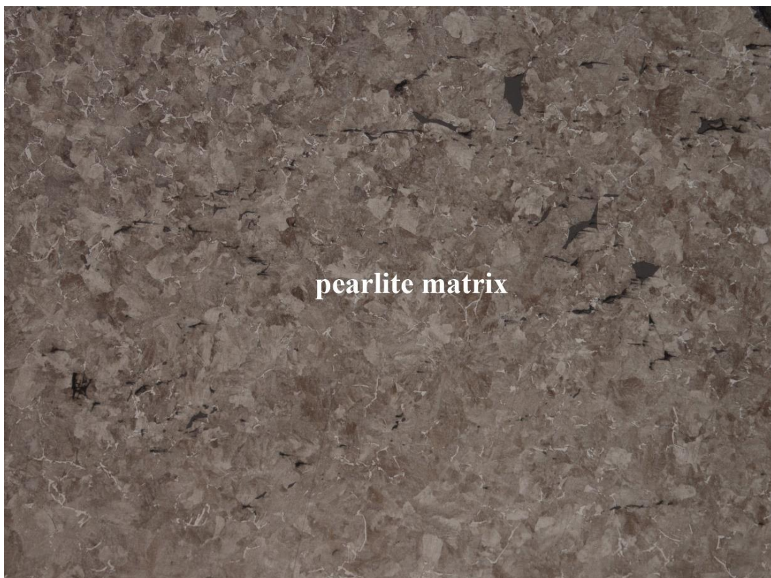
Fig. 5.86 Section from SK0032. Etch 2% nital, scale x37.5 (source: author)
