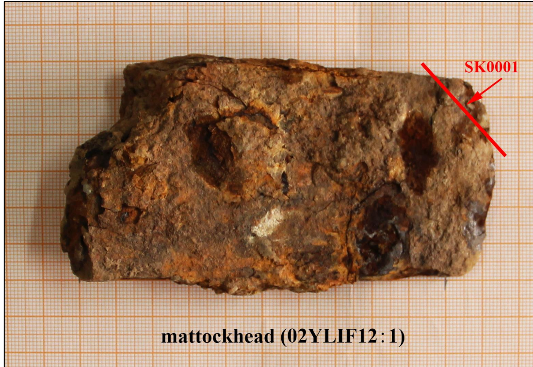
Fig. 5.5 Mattockhead (02YLIF12:1) showing the sampling spot of SK0001 (source: author)
