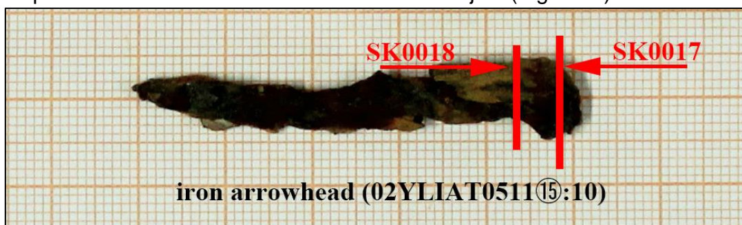
Fig. 5.49 Iron arrowhead (02YLIAT0511(15):10) showing the sampling spot of SK0017 and SK0018 (source: author)
