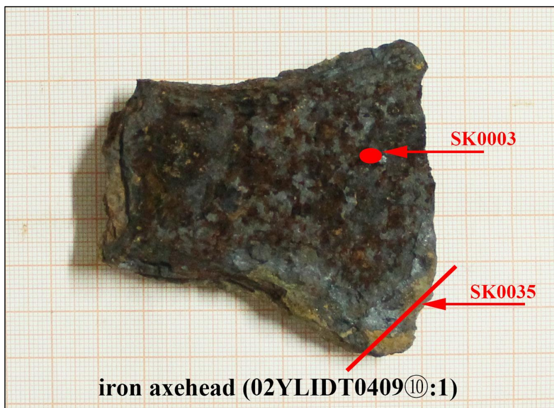
Fig. 5.13 Axehead (02YLIDT0409⑩:1) showing the sampling spot of SK0003 and SK0035 (source: author)
