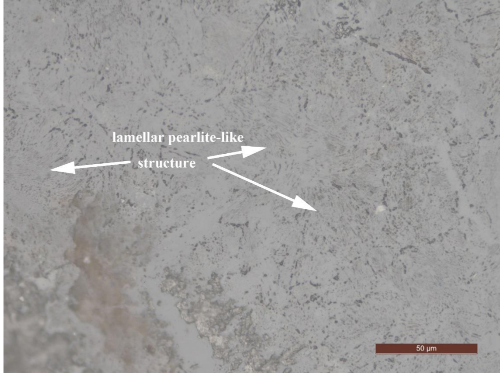
Fig. 5.145 Section from SK0059. Etch 2% nital, scale bar 500μm (source: author)
