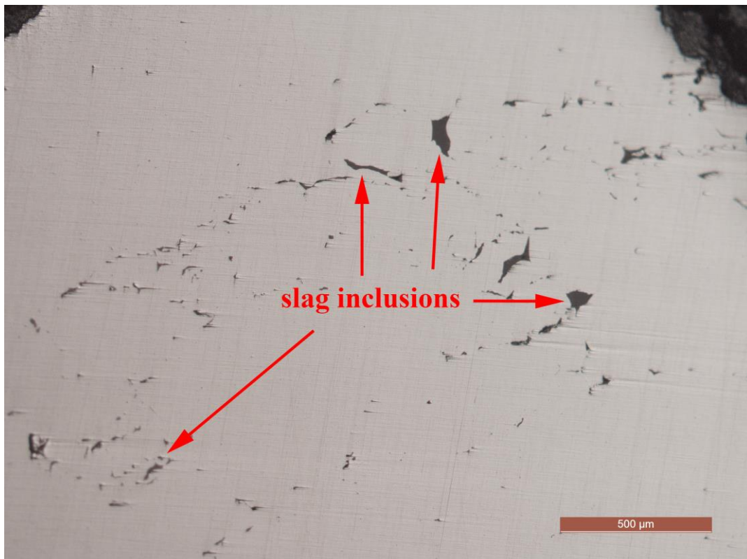
Fig. 5.85 Section from SK0032. Unetched, scale bar 500μm (source: author)
