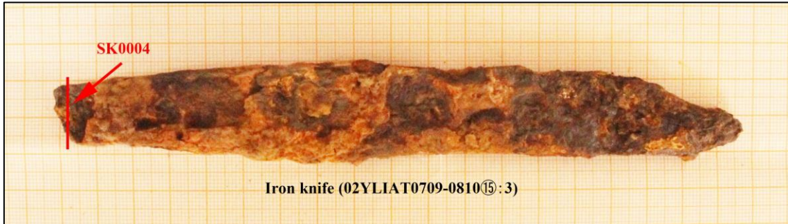
Fig. 5.18 Iron knife (02YLIAT0709-0810⑮:3) showing the sampling spot of SK0004 (source: author)
