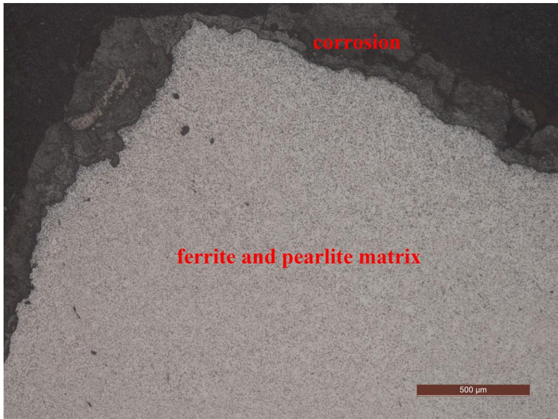
Fig. 5.67 Section from SK0022. Etch 2% nital, scale bar 500μm (source: author)
