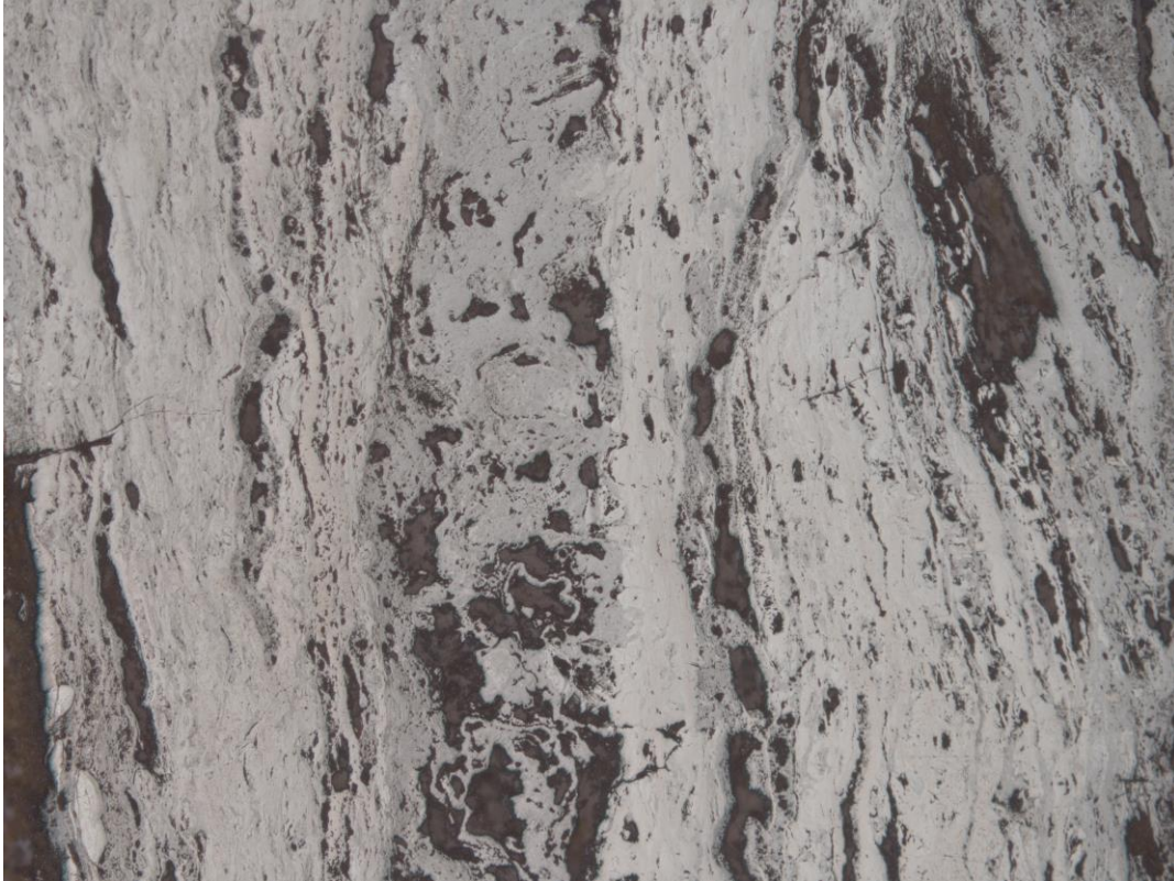
Fig. 5.47 Section from SK0014. Etch 2% nital, scale x37.5 (source: author)
