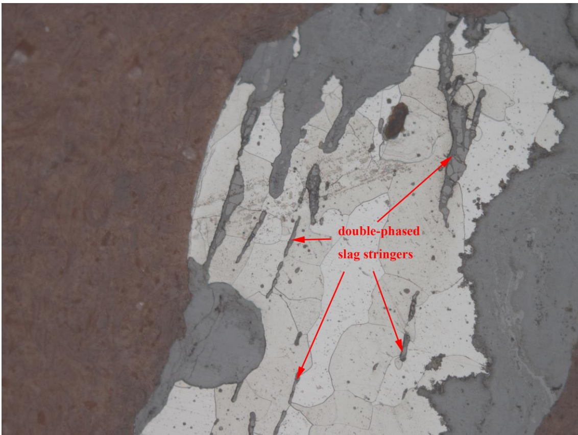
Fig. 5.37 Section from SK0010 showing the double-phased slag stringers. Etch 2% nital, scale x150 (source: author)
