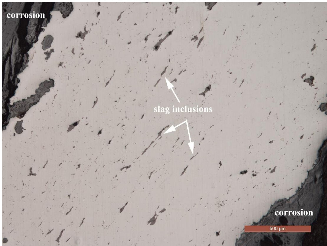
Fig. 5.23 Section from SK0005 showing the slag inclusions. Unetched, scale bar 500μm (source: author)
