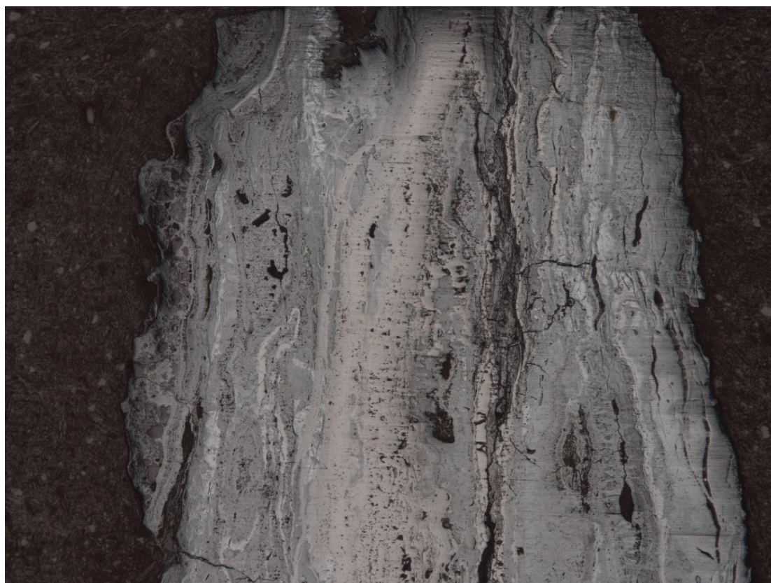
Fig. 5.14 Section from SK0003 showing the corrosion. Etch 2% nital, scale x37.5 (source: author)
