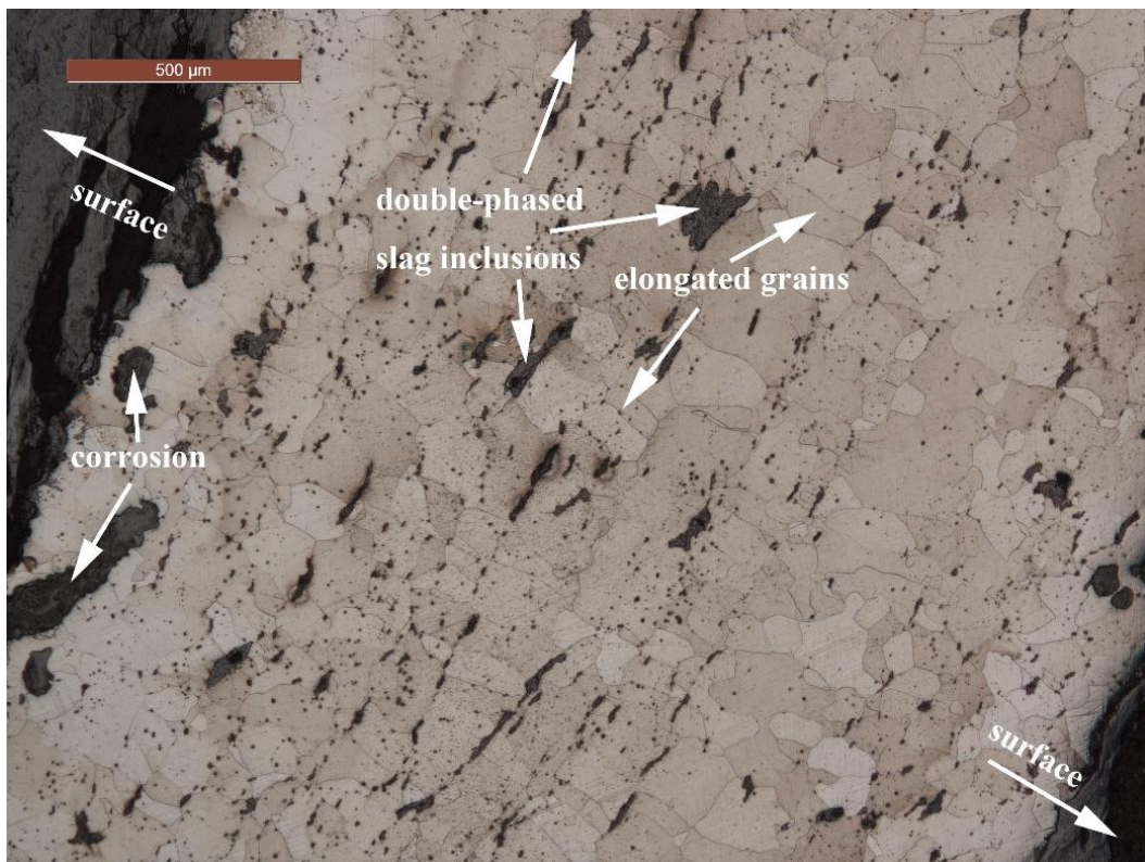
Fig. 5.24 Section from SK0005 showing a ferrite matrix and the slag inclusions. Etch 2% nital, scale bar 500μm (source: author)
