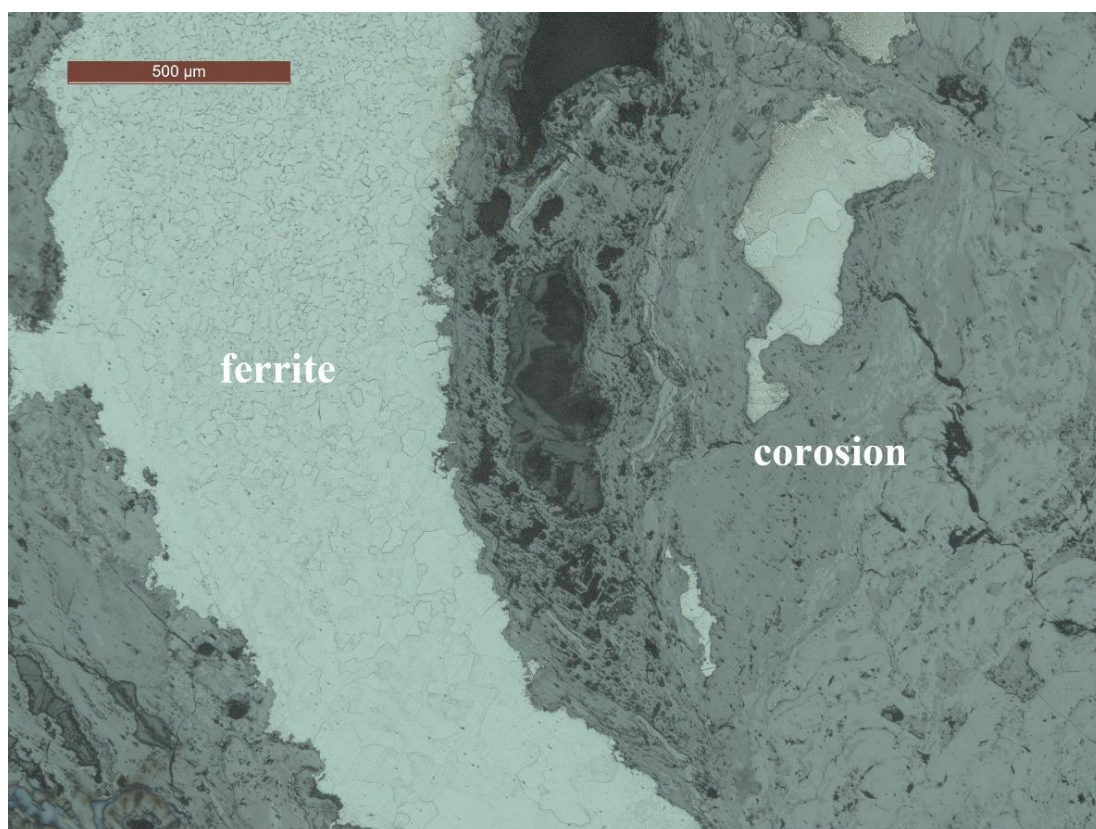
Fig. 5.104 Section from SK0044. Etch 2% nital, scale bar 500μm (source: author)
