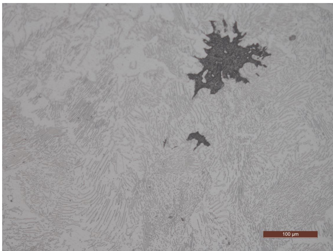
Fig. 5.58 Section from SK0020 showing the lamellar pearlite and the graphite. Etch 2% nital, scale bar 100 \mu m (source: author)
