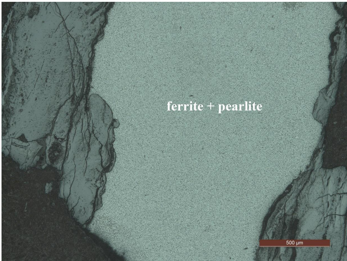
Fig. 5.99 Section from SK0042. Etch 2% nital, scale bar 500 \mu m (source: author)
