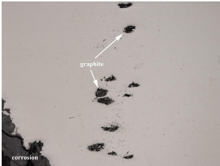
Fig. 5.19 Section from SK0004 showing the metal and the graphite. Unetched, scale x37.5 (source: author)
