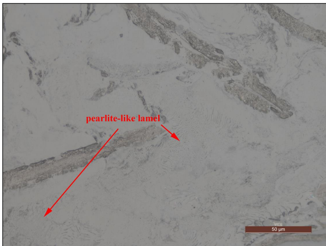
Fig. 3.135 Section from SK0070. Etch 2% nital, scale bar 50μm (source: author)
