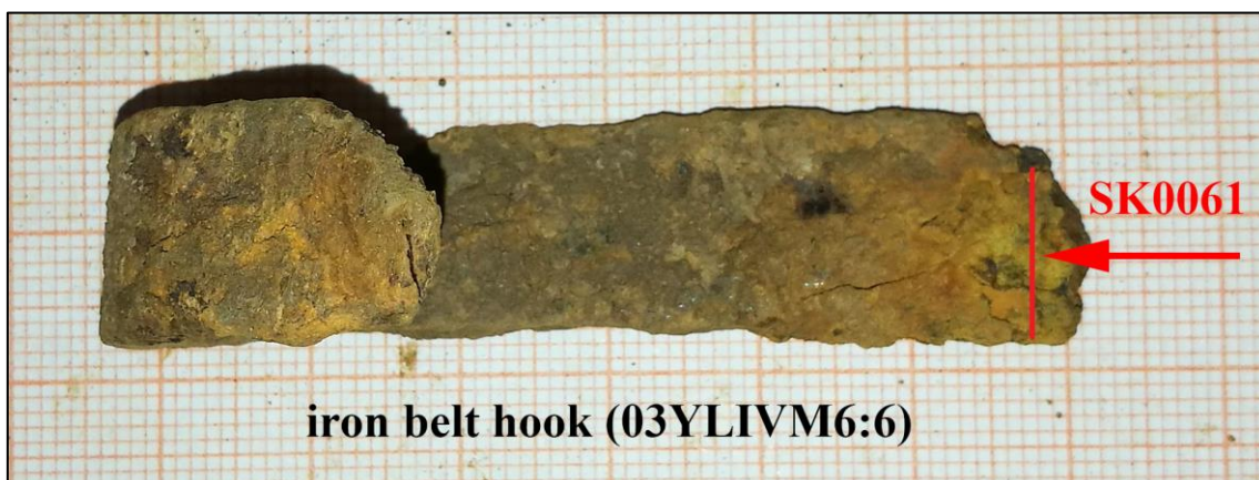
Fig. 5.148 Iron belt hook (03YLIVM6:6) showing the sampling spot of SK0061 (source: author)
