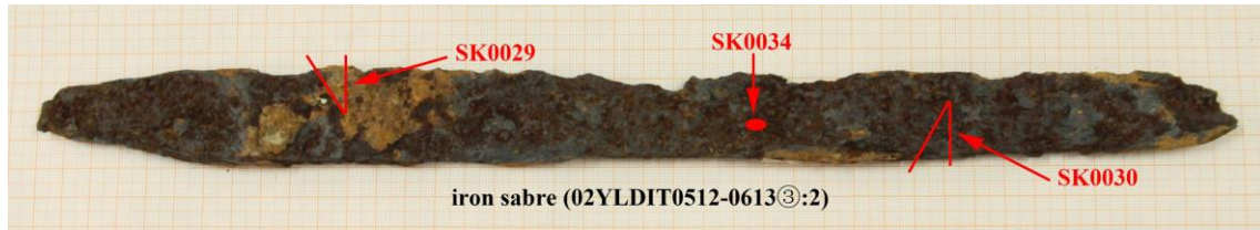
Fig. 5.77 Iron sabre (02YLDIT0512-0613③:2) showing the sampling spot of SK0029, SK0030, and SK0034 (source: author)
