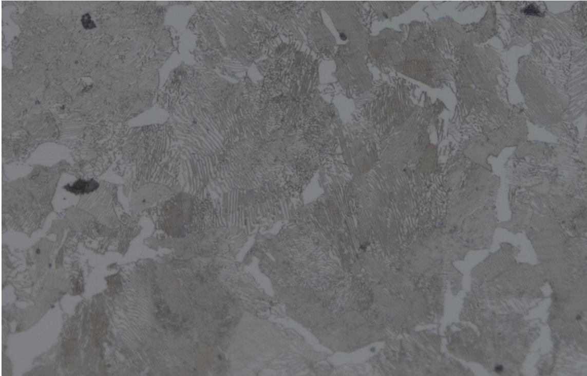
Fig. 5.12 Section from SK0002 showing lamellar pearlite. Etch 2% nital, scale x375 (source: author)
