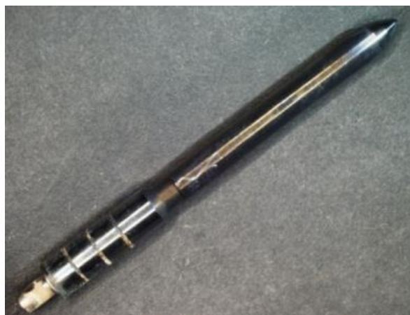
Figure 2.18: Typical appearance of organic amide lacquer deposits 85 .
