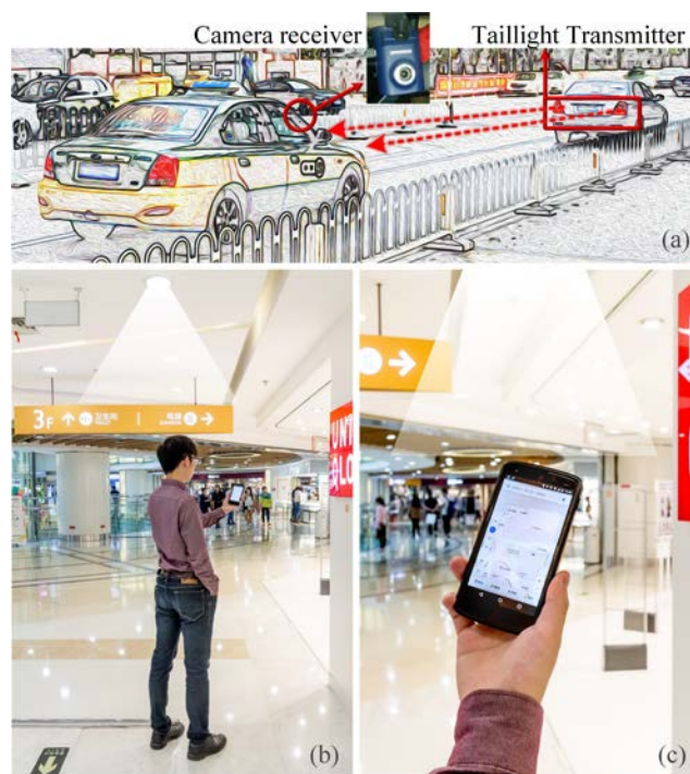
Fig. 1. Scenarios for OCC: (a) V2V communications; (b) indoor positioning; and (c) indoor mapping with real-time location of the user.
