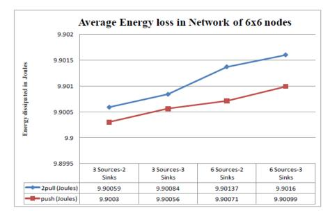
Figure 3-5: The average energy dissipation in 6x6 nodes network
