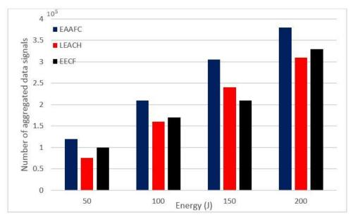
Figure 4-7 The total number of data signals aggregated at the cluster head per given amount of energy
