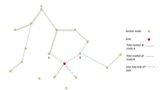
Figure 2-1: Sequential assignment routing. (Rao, et al., 2003, Sept.)
