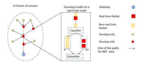
Figure 1-3: Queuing model in cluster-based sensor network, Source: (Akkaya & Younis, 2005)
