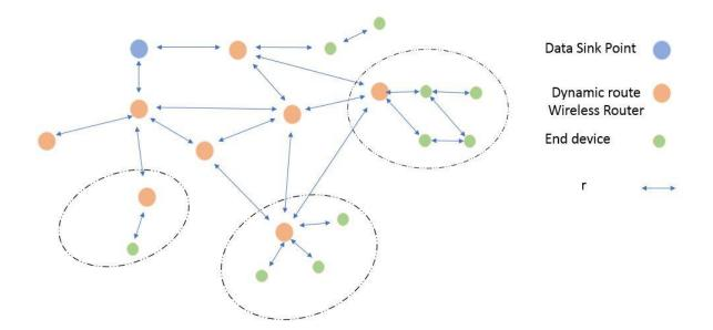
Figure 1-1: C1WSNs: multi point to point, using dynamic routing (Sohraby, et al., 2007)
