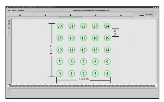
Figure 3-1: Network of 25 nodes in 160 sqm with 40 m distance between nodes in each direction captured in NAM
