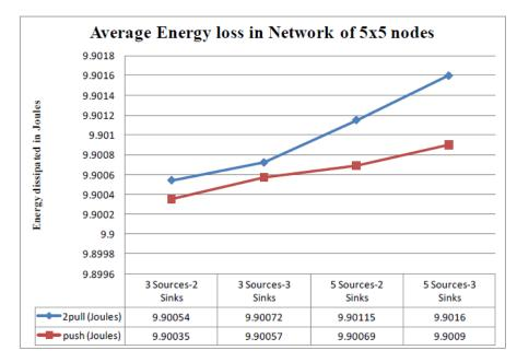
Figure 3-4: The average energy dissipation in 5x5 nodes network
