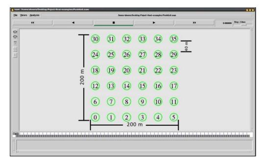
Figure 3-2: Network of 36 nodes in 200 sqm with 40 m distance between nodes in each direction captured in NAM
