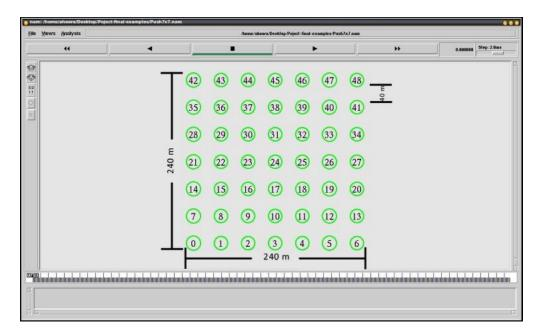
Figure 3-3: Network of 49 nodes in 240 sqm with 40 m distance between nodes in each direction captured in NAM
