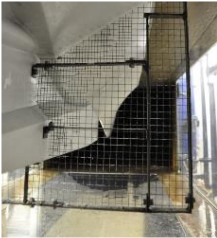
Figure 5: Wake grid fitted to the model hull
