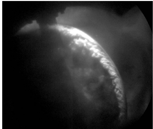
Figure 8: Full-scale cavitation observation at 1200 rpm using a borescope
