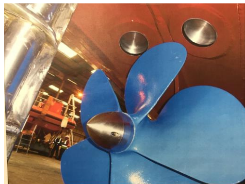
Figure 7: Portholes fitted for the camera observations
