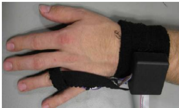
Figure 5 Zigbee-Based Wrist strap prototype connected to a finger ring (Malhi and Mukhopadhyay 2012).
