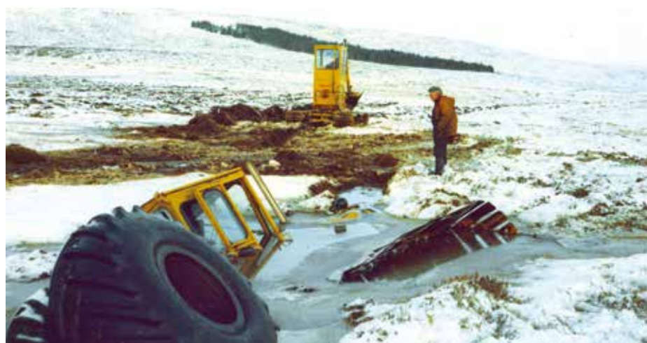
Figure 2: The difficulties of peatland afforestation. In this 1983 image a tractor and plough (the same vehicle as Figure 1) has become bogged down in deep peat at Benmore in Shin Forest, Sutherland. Photograph courtesy of Norman Davidson and http://www.forestry-memories.org.uk .
