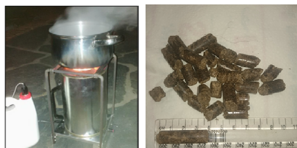
Fig. 1. Photograph of the biomass pellet forced draft cookstove and pellet fuels used. (Photograph: Marian Brown)
