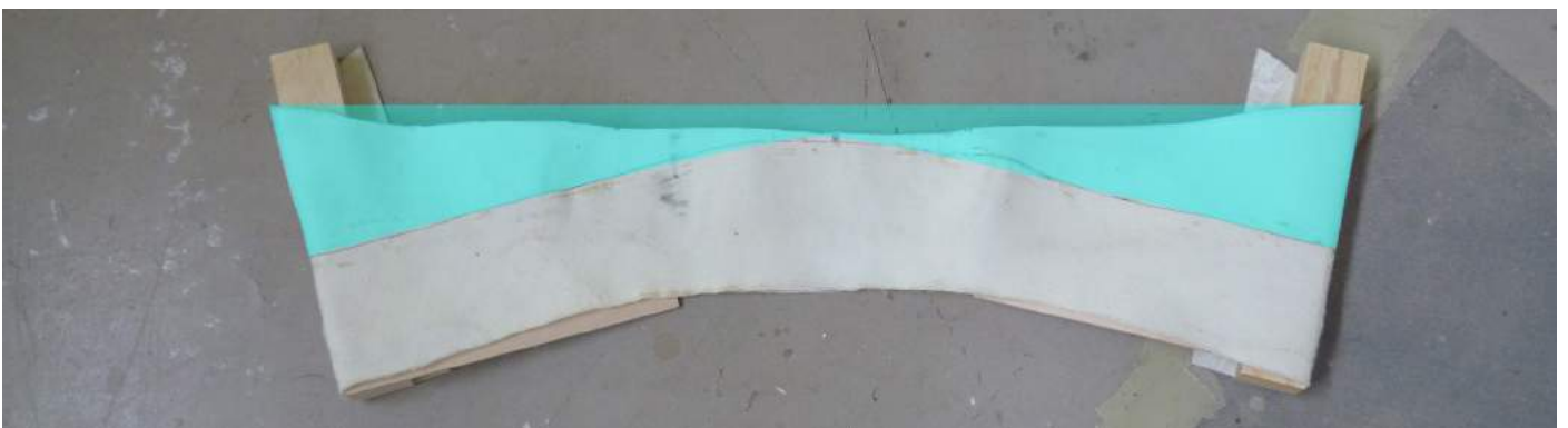
■ More fabrics are added to transfer the pressure from the clamps
