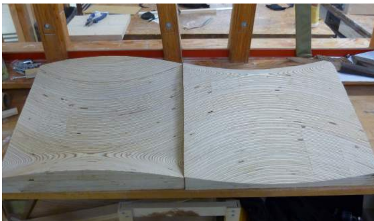
Seat Mould Production by CNC Machine
