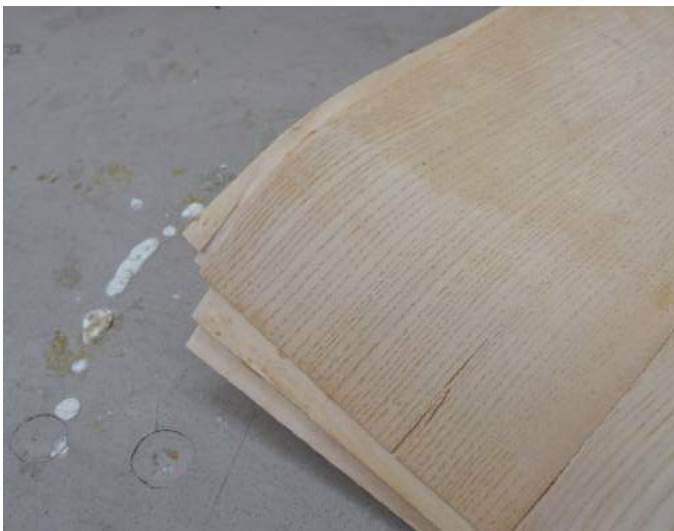
The cracks appear on different veneer direction
