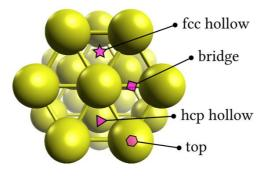
**Figure 7.** Investigated  $BF_4$  adsorption sites at Au(111) surface.
