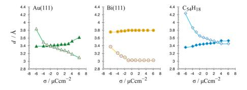
**Figure 14.** Distances (*d*) from top atom layer of Au(111), Bi(111) and  $C_{54}H_{18}$  surfaces to the closest nitrogen atom of cations (filled markers) and boron atom of anions (transparent markers) of EMImBF<sub>4</sub> associates, represented as dependence on the electrode surface charge density.
