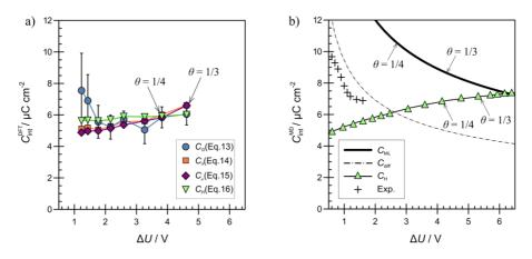
**Figure 10.** a) Dependence of integral capacitance on potential, calculated using the DFT data and Eqs. 13–16. b) Dependencies of integral ( $C_{\text{ML}}$  and  $C_{\text{H}}$ ) and differential ( $C_{\text{diff}}$ ) capacitance on potential calculated using the MD data. Surface coverage values ( $\theta$ ) are labeled with arrows. Experimental data have been taken from Ref. [111], where Au-EMImBF<sub>4</sub> interface was studied using electrochemical impedance spectroscopy.
