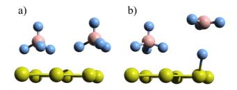
**Figure 6.** a) Au(111) | BF<sub>4</sub><sup>-</sup> interface model at surface coverage  $\theta = 1/3$ . b) BF<sub>4</sub><sup>-</sup> spontaneously dissociates and reorients at the same surface coverage. Only the upper, *i.e.* relaxed layer of gold is shown.
