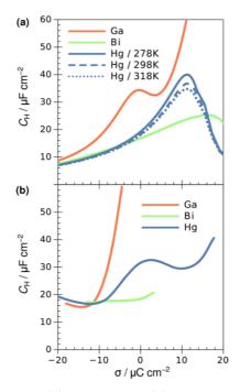
**Figure 3.** (a) Calculated and (b) measured  $C_{_{\rm H}}(\sigma)$  dependencies for Bi(111), Ga and Hg electrodes. The corresponding experimental data are taken from Refs. [39–41].
