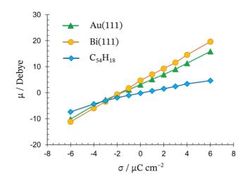
**Figure 17.** Dependence of the dipole moment perpendicular to the surface plane on the surface charge density for interfaces given in Figure 13.
