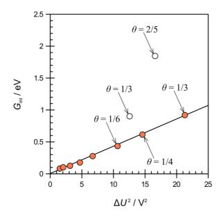
**Figure 8.** Dependence of the integral energy  $(G_{int})$  of  $BF_4^-$  anions (•) on the relative electrode potential squared  $(\Delta U^2)$ . Blank markers ( $\circ$ ) indicate  $BF_4^-$  dissociation to  $BF_3 + F$ . Surface coverage ( $\theta$ ) is labeled with arrows. The slope corresponds to the differential capacitance value of 6  $\mu$ F/cm<sup>2</sup>.
