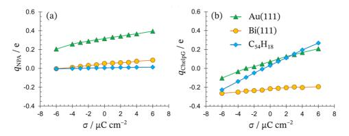
**Figure 16.** Dependence of (a) NPA charge transfer and (b) ChelpG charge transfer values on the surface charge density.
