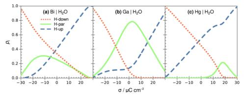
**Figure 4.** Statistical weights  $(p_i)$  of adsorbed water molecules in a given orientation (H-up, H-down, H-par) depending on the electrode surface charge density, calculated for (a) Bi(111), (b) Ga and (c) Hg electrodes.
