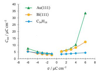
**Figure 18.** Dependence of the integral capacitance on the surface charge density for interfaces noted in Figure 13.
