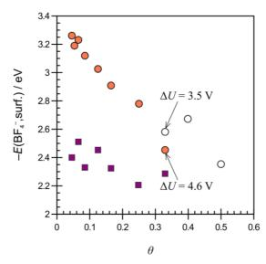
**Figure 9.** Dependence of the  $BF_4^-(\bullet)$  and  $F^-(\bullet)$  adsorption energies  $(E_{ads})$  on the surface coverage. At high coverage,  $BF_4^-$  is oxidized and dissociates into  $BF_3$  and  $F^{\cdot}(\circ)$ . Relative electrode potential  $(\Delta U)$  is labeled with arrows.
