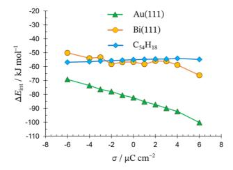
Figure 15. Dependence of interaction energy on the surface charge density.
