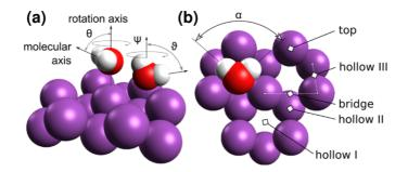
**Figure 2**. (a) Side and (b) top views of different adsorption sites at the model metal clusters used to describe the adsorption of  $H_2O$  molecule at a Bi(111) surface cluster. The bond angle  $\alpha$  characterizes the internal geometry of the molecule, and the rotation angles  $\theta$ ,  $\psi$  and  $\vartheta$  characterize orientation of the molecule relative to the surface normal labeled as "rotation axis".
