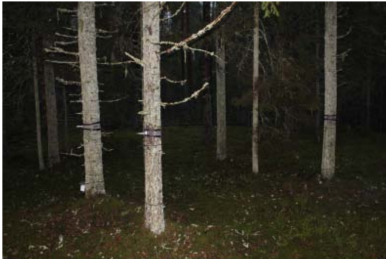
Photo 2. Dendrometer on sample trees
