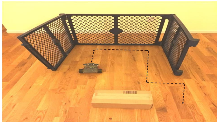
Figure 6. The trajectory of the robot when detecting a U-shaped obstacle.
