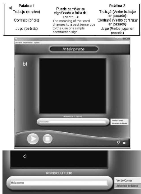
Figure 4: From up to down: (a) Change of meaning in the word according to accentuation sign. (b) current banner for unknown sign, (c) Sentence selection in the case of homonym and homograph word. In (b) the SLI system is programmed to detect homonym words on the database by showing a current banner. The desired meaning for the sentence or word is given to be chosen afterwards.
