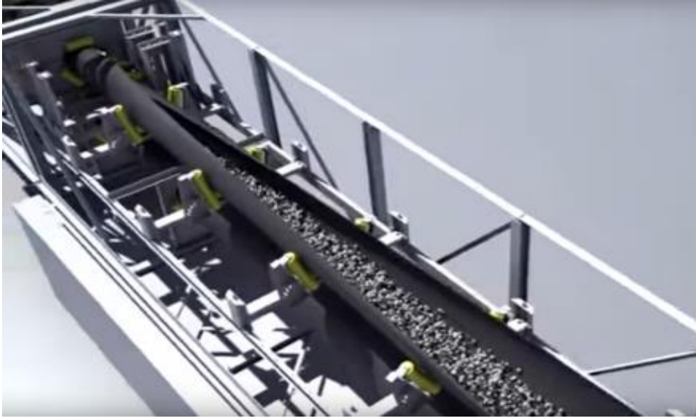
Figure 6. Pipe conveyor system showing the rolling phase.
