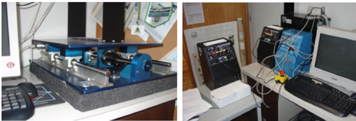
Figure 15. Quanser shaking table II (and its controllers) at FEUP – COVICOCEPAD Lab.
