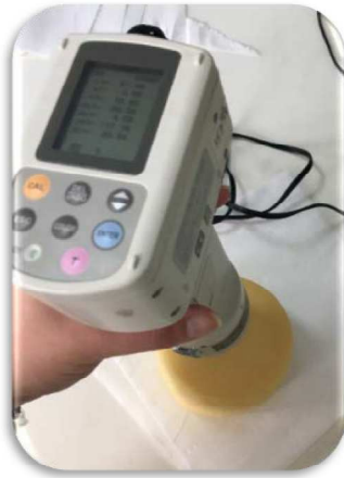
Figure 2. Example of a colour measurement of cheeses.
