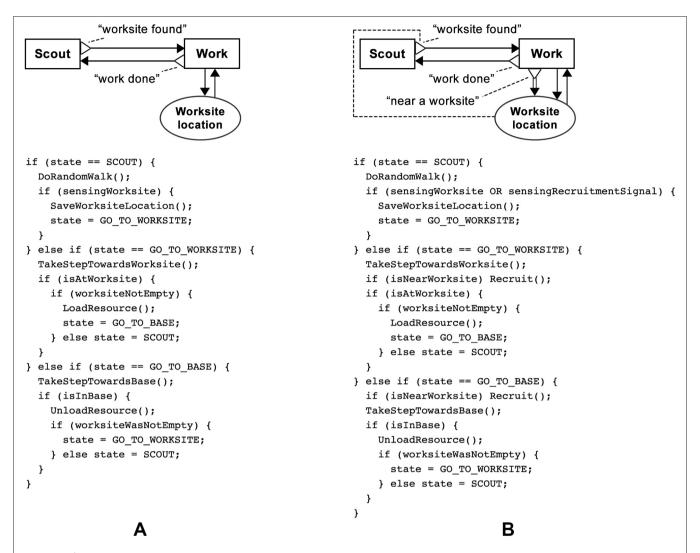
FIGURE 12 | (A) Graphical BDRML representation of the "Solitary" robot control algorithm, resulting from the Individualist design pattern, and robot update loop pseudocode. (B) Graphical BDRML representation of the "Local Broadcaster" robot control algorithm, resulting from a combination of the Broadcaster and Information Exchange near Worksites patterns, and robot update loop pseudocode.
