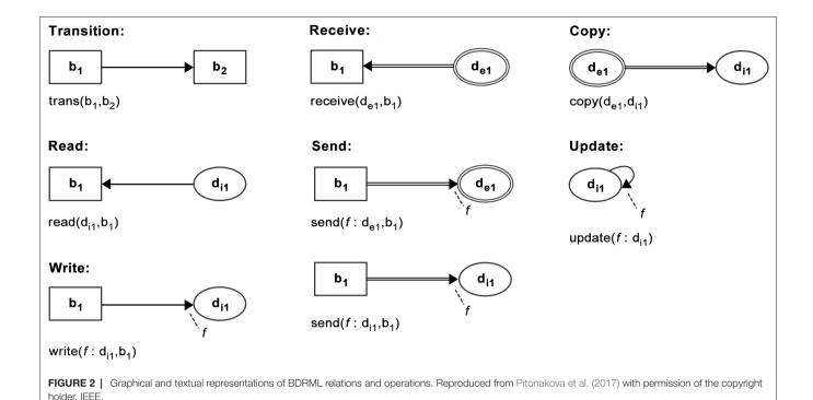
• *Update:* The value of a data structure is updated from that in the previous time step by a subroutine not visualised in the BDRML diagram (for example, a pheromone level may "spontaneously" decrease over time).
