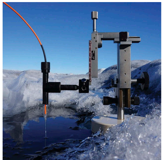
Figure 3. Microoptode positioned with a manual micromanipulator for in situ measurement of an oxygen profile in a cryoconite hole on the surface of the Greenland Ice Sheet.
