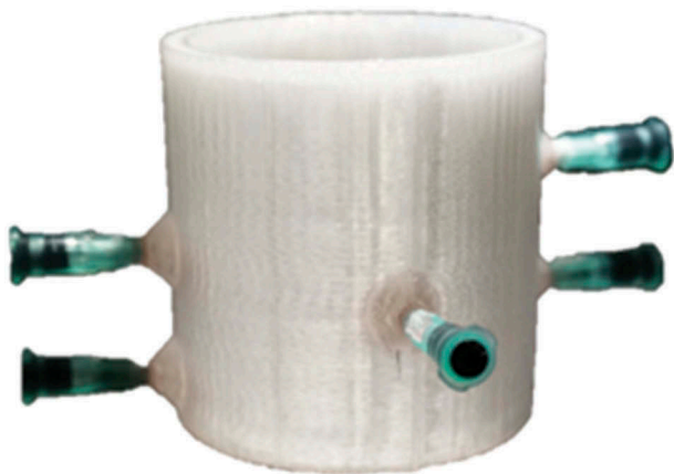
Figure 2. A custom-made incubation vessel, manufactured using 3D printing with sampling ports on the sides to enable measurement of oxygen, pH, and microbial community changes with depth.
