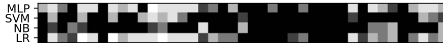
FIG 16. The beta calibration test p-values of MLP, SVM, NB and LR (4 rows) per dataset (41 columns). Each p-value has been averaged over all cross-validation folds. The greyscale colours represent the same bins as in Figure 15, with white standing for negative logarithm p-value below 1 and black for above 5 (very significantly not calibrated). The order of datasets in the columns is the same as in Table 1.
