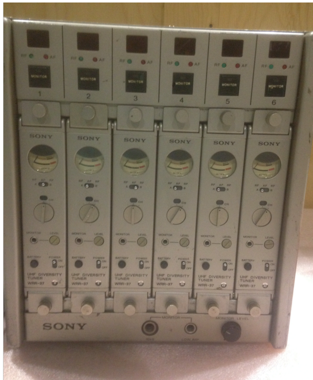
Fig. 19: Sony WRR UHF diversity radio mic receivers. (Image: Tim Heath)
