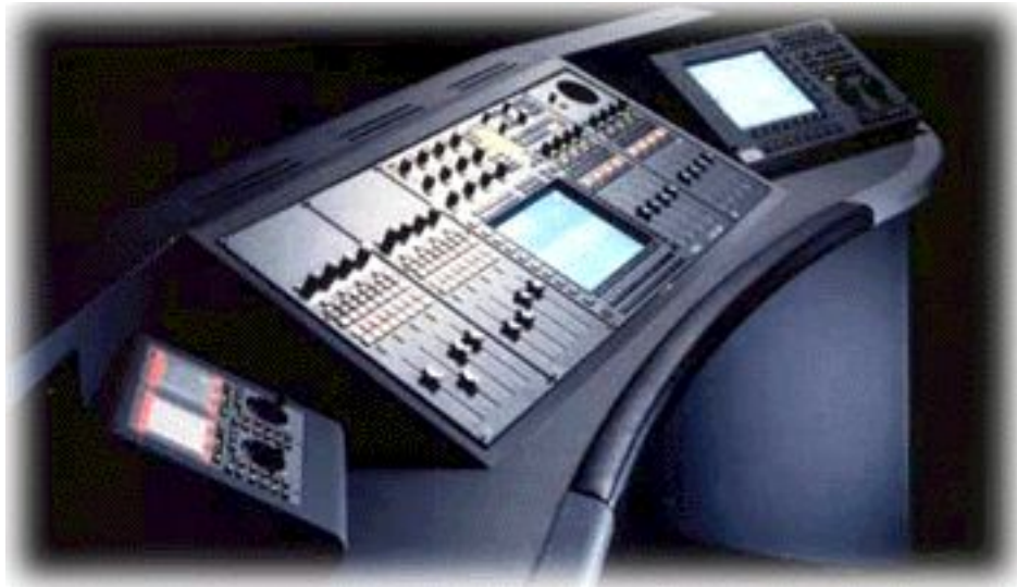
Fig. 16: AMS Logic 3 DAW station, incorporating Audiofile (Image: AMS-Neve, 2017)
