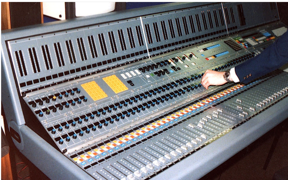
Fig. 20: Neve DSP - the world's first fully digital desk (Image: Pro Audio Europe, 2017)
