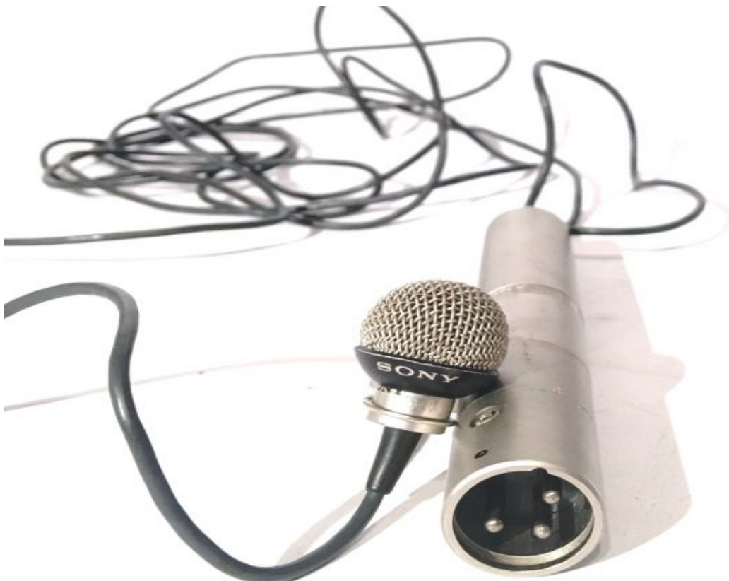
Fig. 7: Sony ECM 50 microphone including battery pack and XLR connector (Photo: Vintage Tools, 2017)
