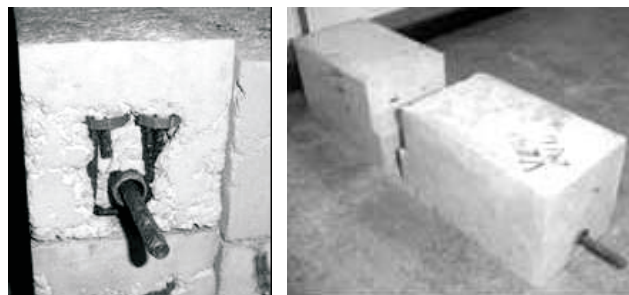
Figure 15– Beam specimen with los fluidity (right) and specimen with best fluidity (left)
