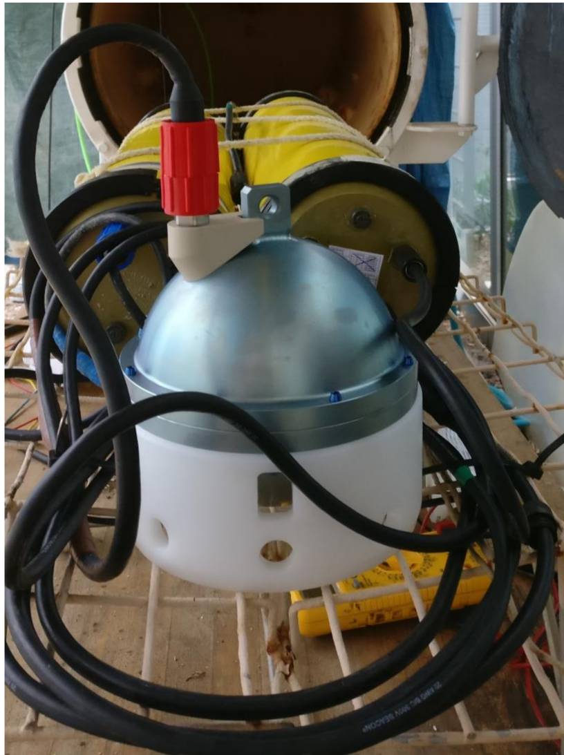
Figure 3. The Ocean Bottom Seismometer (OBS) with Güralp 6TC seismometer at pressure test. The bottom case of the seismometer is grooved to evacuate exceeding material for a successful coupling with the seafloor.
