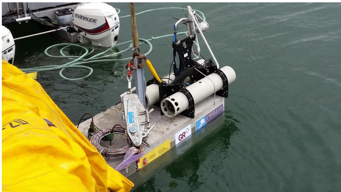
Figure 2. The prototype ocean bottom broadband unit.
