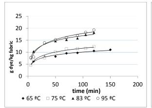
**Figure 7** Kinetics of dyeing with C.I. Disperse Blue 56 absorbed by polyester fabric at different temperatures in the presence of butyl acetate (16.666  $g \cdot l^{-1}$ ) and coumarin ( 0.666  $g \cdot l^{-1}$ ).
