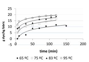
**Figure 8** Kinetics of dyeing with C.I. Disperse Blue 56 absorbed by polyester fabric at different temperatures in the presence of butyl acetate (16.666  $g \cdot l^{-1}$ ) and *o*-vanillin (0.666  $g \cdot l^{-1}$ ).
