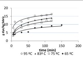
**Figure 5** Kinetics of dyeing with C.I. Disperse Red 73 absorbed by polyester fabric at different temperatures in the presence of butyl acetate (16.666  $g \cdot l^{-1}$ ) and coumarin (0.666  $g \cdot l^{-1}$ ).
