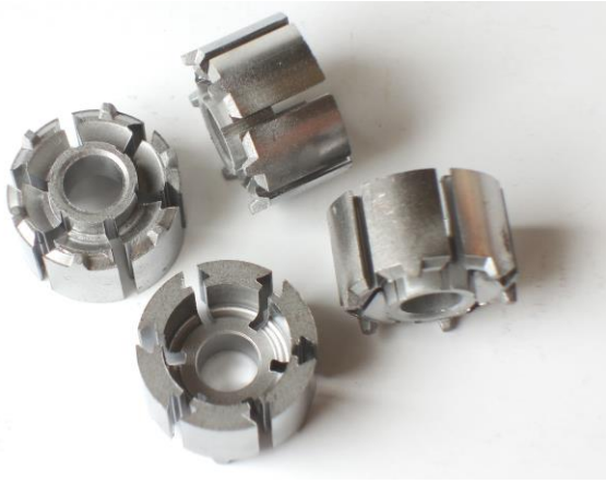
Figure 6: Pure iron parts used in an electromagnetic disk brake in a home automation system
