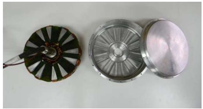
Fig. 13 Stator and the two covers, showing in the middle cover the SMC rotor pole pieces mounted
