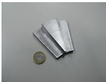
Fig 6 Stator pole (up) and rotor pole pieces (down) made of SMC
