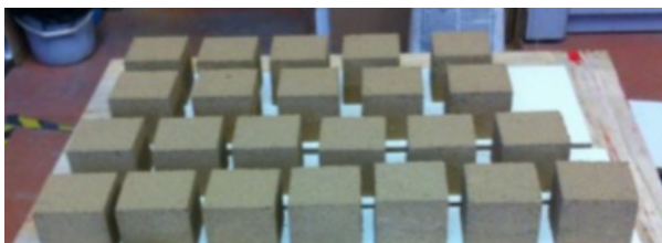
FIGURE 2. Specimens 2CA and 4CA, and three additional specimens with no bacteria to control the evolution of the moisture content.
