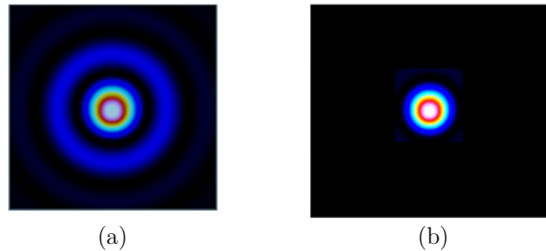
Figure 2.12 Airy pattern obtained by a (a) conventional microscope and a (b) confocal microscope. Source: [58]
