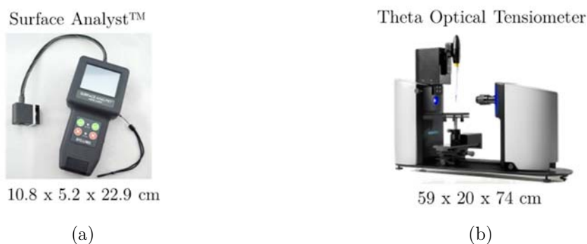
Figure 2.24 Representative devices from Dyne Testing. (a) Portable device for measuring the contact angle. (b) Laboratory device for measuring the contact angle, surface energy of a solid and the interfacial tension.
