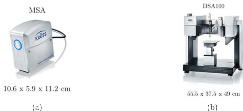
Figure 2.22 Representative devices from KRÜSS to measure the contact angle and the surface energy of a solid by means a (a) portable device and (b) Laboratory device.
