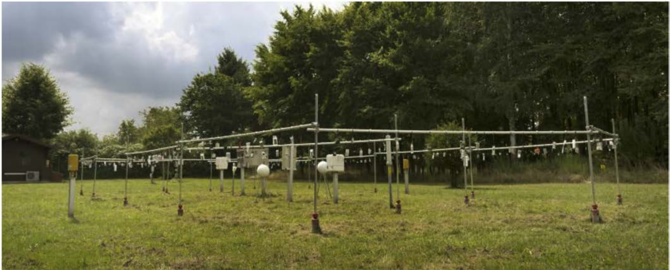
Fig. 1. Dosimeters exposed at the PTB reference site for environmental radiation.
